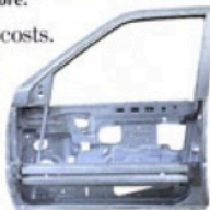
Side doors are reinforced with high-strength steel beams that help protect vehicle occupants in the event of a side impact.
