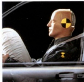
Concealed in the steering wheel, the driver's side air bag inflates within 50 milliseconds and activates when a front-end collision occurs at speeds of 19 kph or more.
