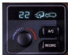
The Automatic Temperature Control system on Grand Cherokee Limited lets you select a degree setting and forget it. Grand Cherokee employs R-134a air conditioning refrigerant, identified as non-hazardous to the ozone layer.
